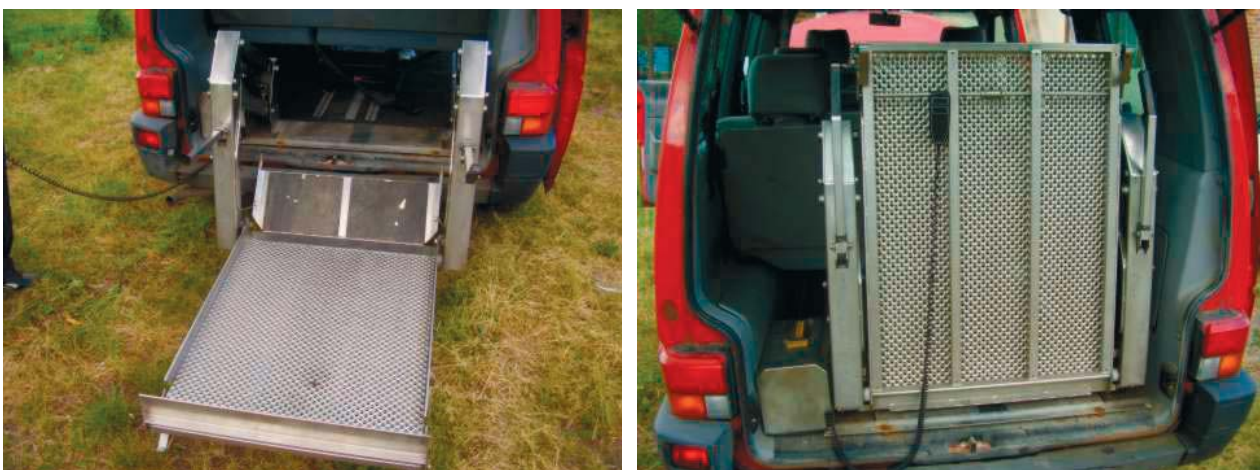
Fig. 1. The lift in raised and lowered position
