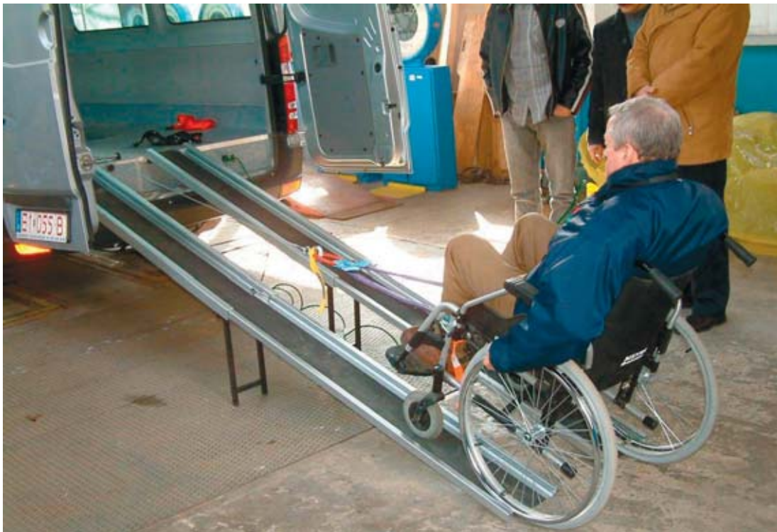
Fig. 2. The outlook and way of using bus- bars and winch in the bus
